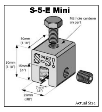
The S-5-E and S-5-E Mini clamps are each furnished with the hardware shown above. Each box also includes a bit tip for tightening setscrews using an electric screw gun. A structural aluminum attachment clamp, the S-5-E is compatible with most common metal roofing materials excluding copper. All included hardware is stainless steel. Please visit www.S-5.com for more information including CAD details, metallurgical compatibilities and specifications.
