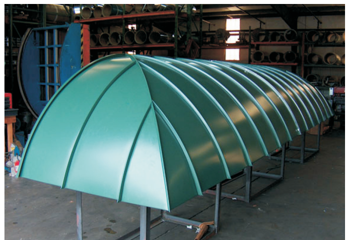
A barrel vault canopy for a restaurant in Florida. The roof panels are 24ga galvalume steel, using our 1" batten seam roof panels and caps. Our customer supplied his aluminum frame for this project. Note the seam caps at the hip.
